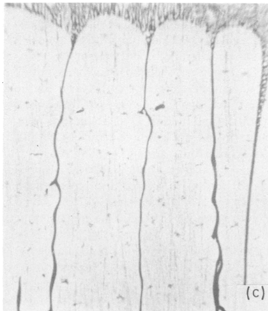
Figure 1 Photomicrographs of longitudinal sections of directionally solidified and interface-quenched Al-4 wt % Cu dendritic monocrystals pulled at 0.30 \text{ m h}^{-1} , \times 100 . Holding times prior to quenching were: (a) 0, (b) 150 and (c) 900 sec.
